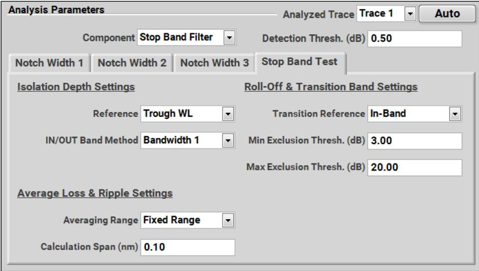
The screenshot shows the **Analysis Parameters** dialog box for a **Stop Band Filter** component. The **Analyzed Trace** is set to **Trace 1** and the **Auto** button is visible. The **Component** is set to **Stop Band Filter** and the **Detection Thresh. (dB)** is **0.50**. The **Stop Band Test** tab is selected, showing the following settings:
