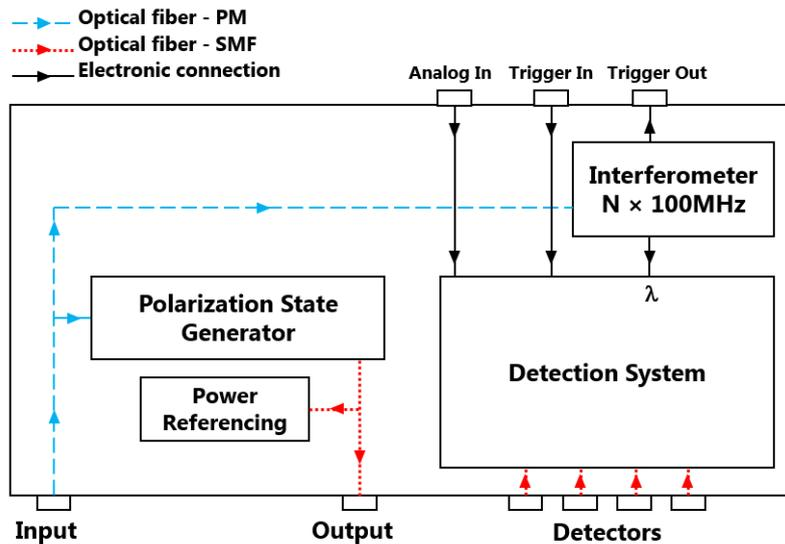
On CT440 with PDL option, the signal passes through a polarization state generator (PSG) that produces one of 6 states of polarization at the output port.
