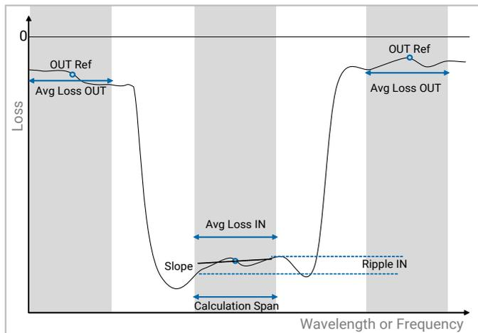
➤ **% Bandwidth:** sets the range to a fraction of the bandwidth measured from the **Notch Width 1** tool (see *Spectral Width x Results* on page 77).
