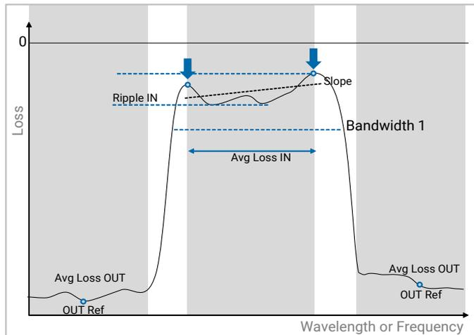
In-band and out-band average loss and ripple/slope calculations are performed across a given calculation span centered on their respective reference points as defined in crosstalk settings.
