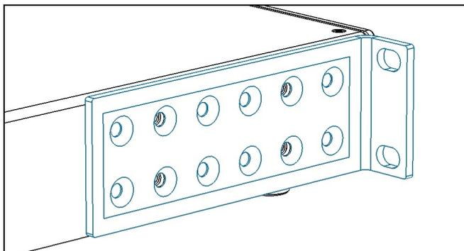
3. Attach the bracket to the side panel with the four 8 mm screws provided with the bracket, using a phillips head screwdriver.
