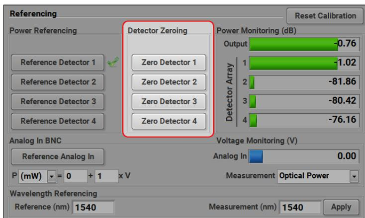
3. In the **Referencing** window, click the **Zero Detector** button corresponding to the wanted detector.
