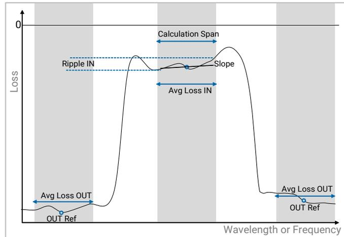
➤ **% Bandwidth:** sets the range to a fraction of the bandwidth measured from the **Spectral Width 1** tool (see *Spectral Width x Results* on page 77).
