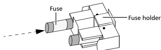
5. Make sure the fuses are placed firmly in the holder prior to reinsertion.
