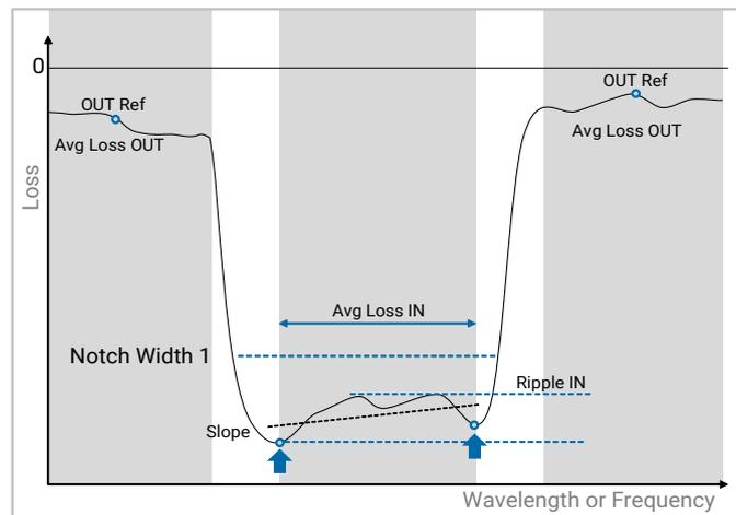
In-band and out-band average loss and ripple/slope calculations are performed across a given calculation span centered on their respective reference points as defined in isolation depth settings.
