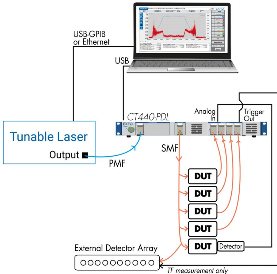
One to four optical detectors enable the CT440 to provide the direct TF and PDL (if available) of the DUT.
