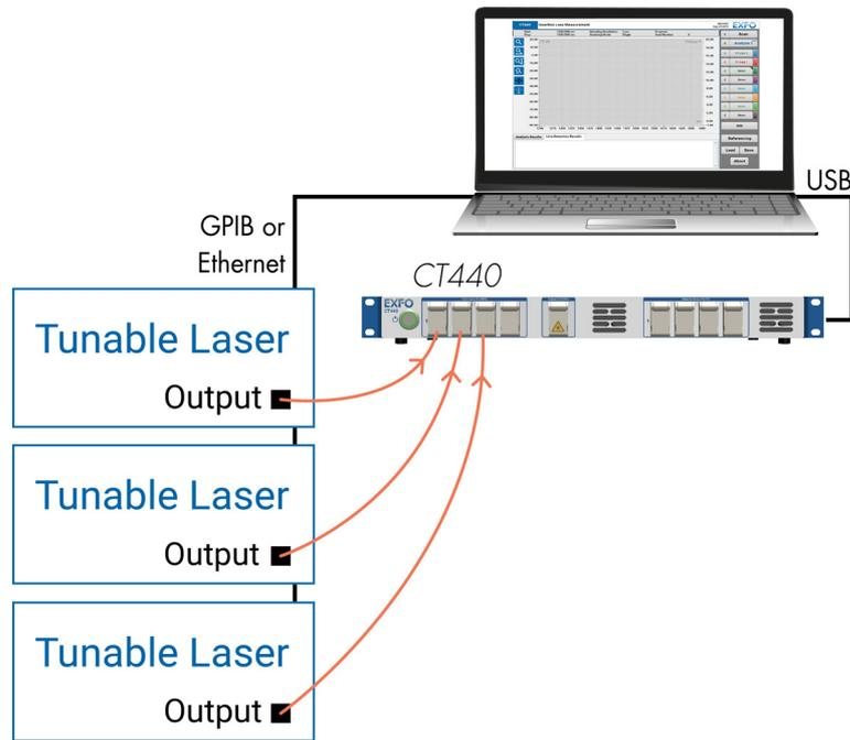
The following figure illustrates the connection of a CT440 with PDL option to a laser.
