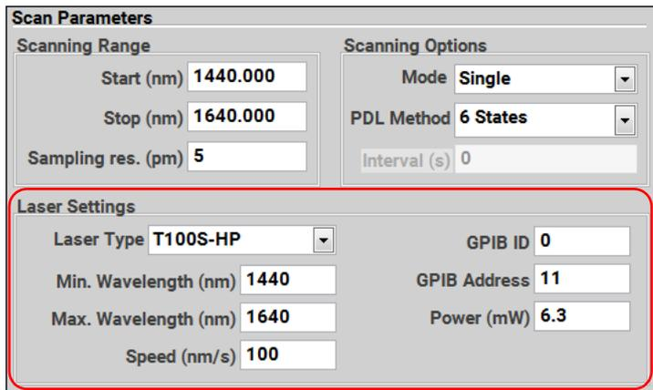
3. Set parameters for the laser(s) connected to the CT440 (1 tab per connected laser), according to the instructions given in the following table.
