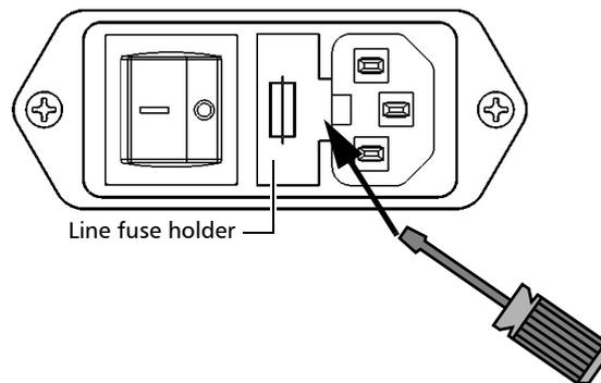
3. Check and replace the fuses if necessary.
