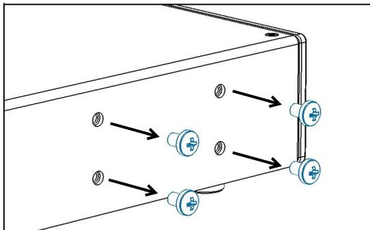
2. Position the left-side bracket on the side panel so that you see the screw holes on the side panel, and it is flush with the front panel of the instrument.
