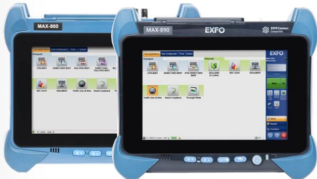
Easy-to-use and portable, the EtherCHK testers include all the test options needed to test **RFC 2544** and **EtherSAM (Y.1564)**. The kit also includes **EtherBERT, traffic generation and monitoring (TGEN)** and dual-port testing.
