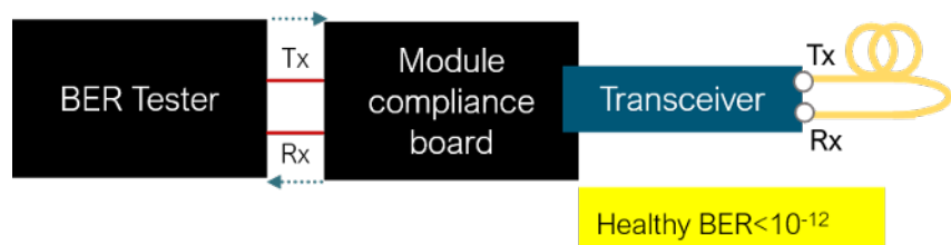
Figure 4. Typical setup to run a BER test of an optical transceiver
