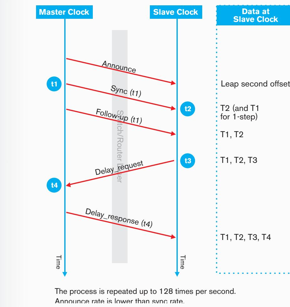
$$\text{Round-Trip Delay (RTD)} = (T_2 - T_1) + (T_4 - T_3)$$
