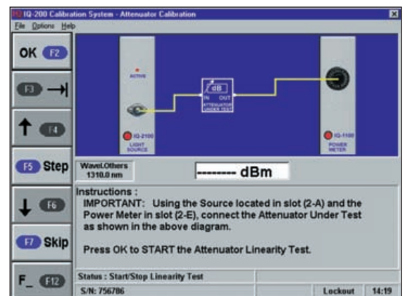
■ Optical attenuation linearity test setup
