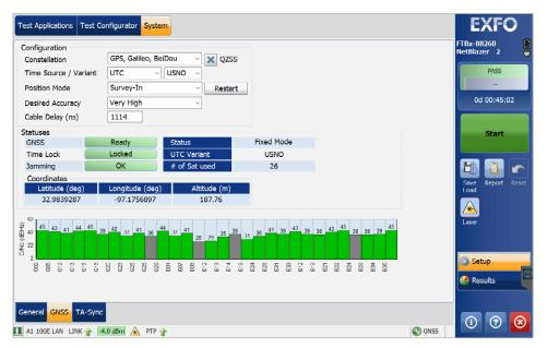
Figure 5. Integrated GNSS configuration and statuses user interface.
