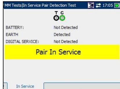
**Note:** *Test beeps or warns when ground is NOT present or very poor.*
