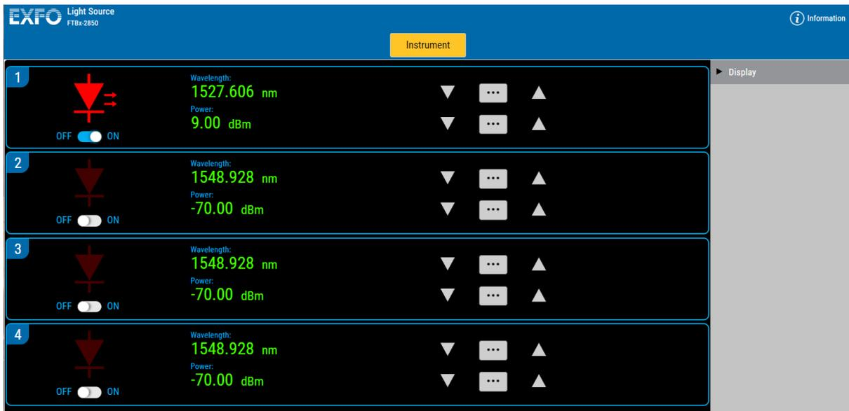
If the installed module features multiple optical sources, you can select which ones are displayed.
