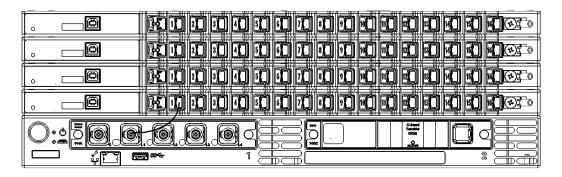
**Note:** Since the RTUe-9120 switch is equipped with unpinned MPO ports (two rows of eight fibers each), you will need a patchcord with a pinned MPO connector.
