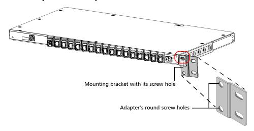
**Note:** To better suit your installation needs, you can flip the orientation of the adapter, as long as you use one of its round holes to attach it to the mounting bracket.
