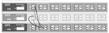
**6.** If your primary switch is a single channel width switch having 52 ports, repeat step 5 with the remaining switches that you want to cascade (up to two more switches).
