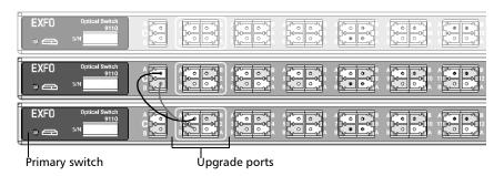
**Note:** The common port(s) of the primary switch are used to receive the signal from a test module.
