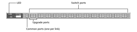
**Note:** On all RTUe-9110 models shown above, you can use the upgrade ports to cascade external switches, or use them as standard switch ports. The upgrade ports have lower insertion loss (IL) than the other ports, which makes them particularly well suited for switch cascading.
