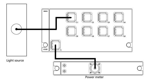
**4.** The IL registered on the power meter will then be the switch port IL including connectors.
