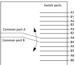
1 x N Duplex Optical Switch Principle
