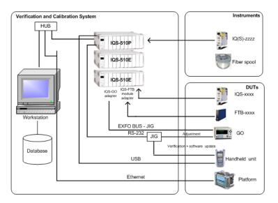
The required instruments vary according to the DUTs and the type of verification and adjustment you want to perform.
