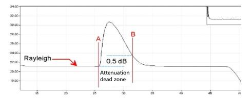
Marker A is positioned at the rising edge of the reflective event. Marker B is positioned within the falling edge, 0.5 dB above the backscatter level.
