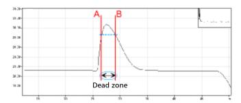
Markers are positioned on both side of the peak,  $1.5~\mathrm{dB}$  below the maximum peak value.
