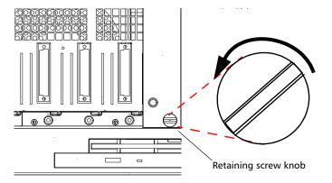
**2.** Place your fingers underneath the module or hold it by the retaining screw knob (*NOT by the connector*) and pull it out.
