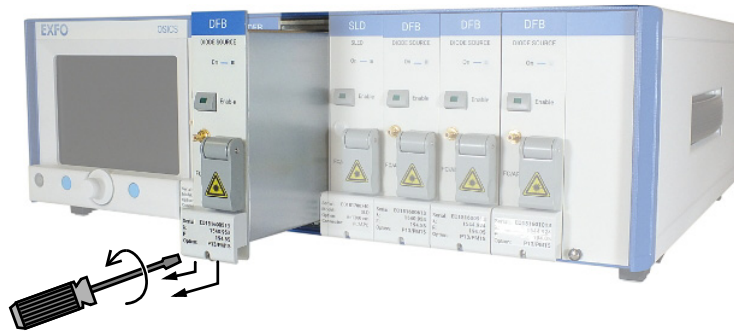
Figure 6: Module Installation – Module Removal
