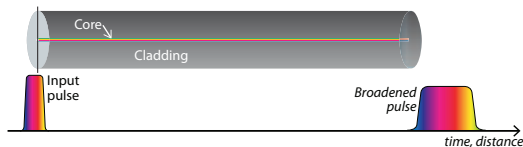
Diagram 4 – Intramodal chromatic dispersion of a single-mode optical fiber
