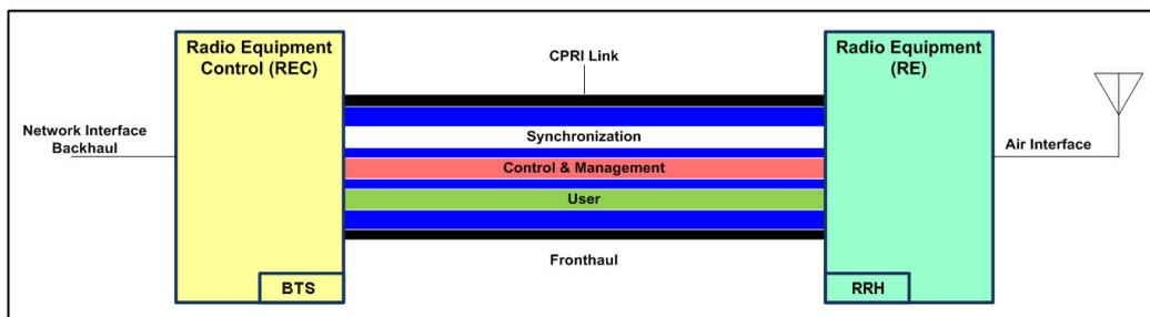
An electrical link is also available from CPRI but it is typically used for base station shelf interconnection. Since a state machine drives the link parameters (rates, protocol, and C&M channel) alignment, a BTS (defined as Master in the standard) and RRH (defined as Slave in the standard) interfaces are defined where the Master initiates the negotiation procedure necessary to achieve this alignment.
