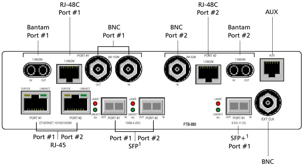
1. Laser radiation emitted from this port when LASER LED is on.
