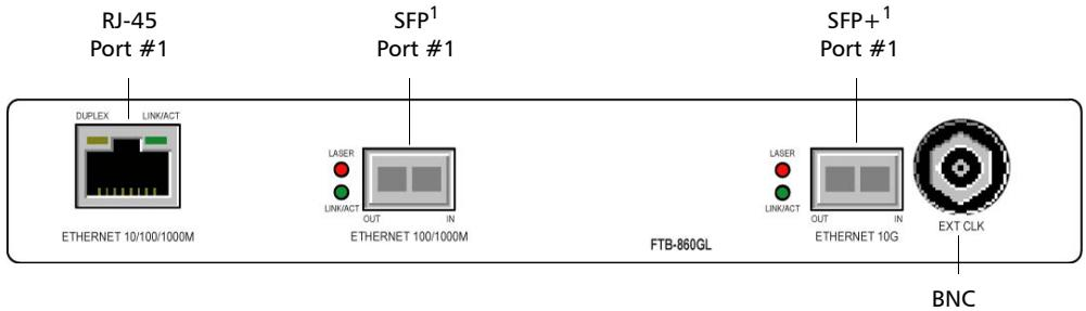
1. Laser radiation emitted from this port when LASER LED is on.
