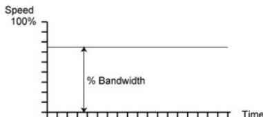
**Burst** transfers the selected frame at maximum bandwidth for the selected **Burst Duty Cycle** over the **Period**.
