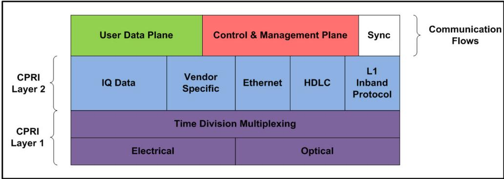
The User Data Plane contains mostly voice/data traffic in the form of IQ Data samples. IQ Data digitally encodes the change in amplitude/phase of a user device modulated signal sampled at the RE antenna.
