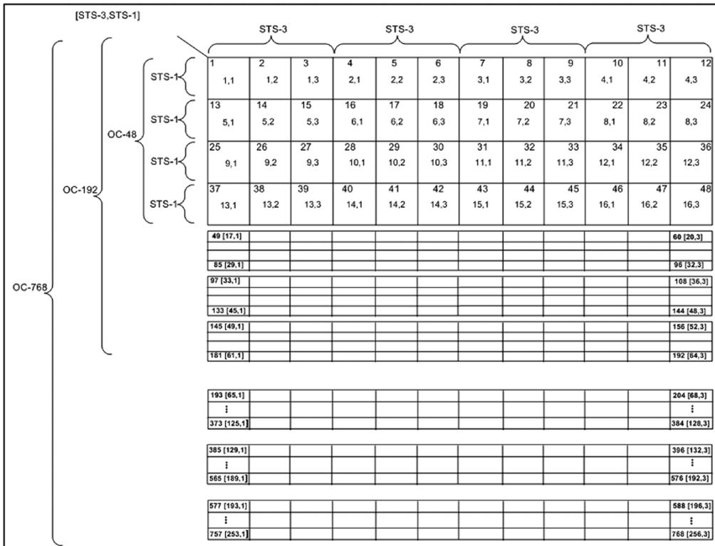
The FTB-700G/800 Series supports numbering SONET low order path using the two-level “VTGroup#,VT#” convention for numbering VTs within an STS-1. For example: VT1.5 [1,3], VT2 [3,2], VT6 [6,1].
