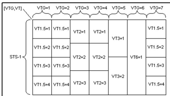
The FTB-700G/800 Series supports numbering SONET high order path STS-nc within an OC-N using the two-level “STS-3#,STS-1#”. For example: STS-12c [5,1].
