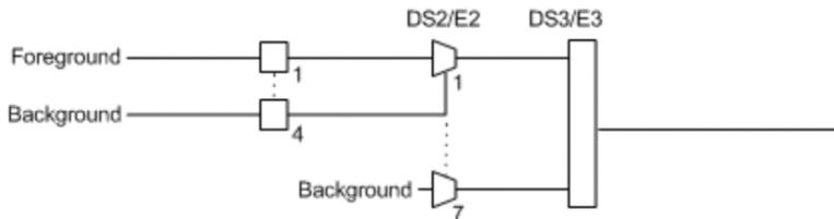
The diagram above shows a test case defined with DSn/PDH traffic where the background traffic is also inserted for the unused timeslots in a test case data path. The insertion is similar to the low order path SONET/SDH terminated signal where the background traffic format inserted uses the same rate as the one defined in the test case data path.
