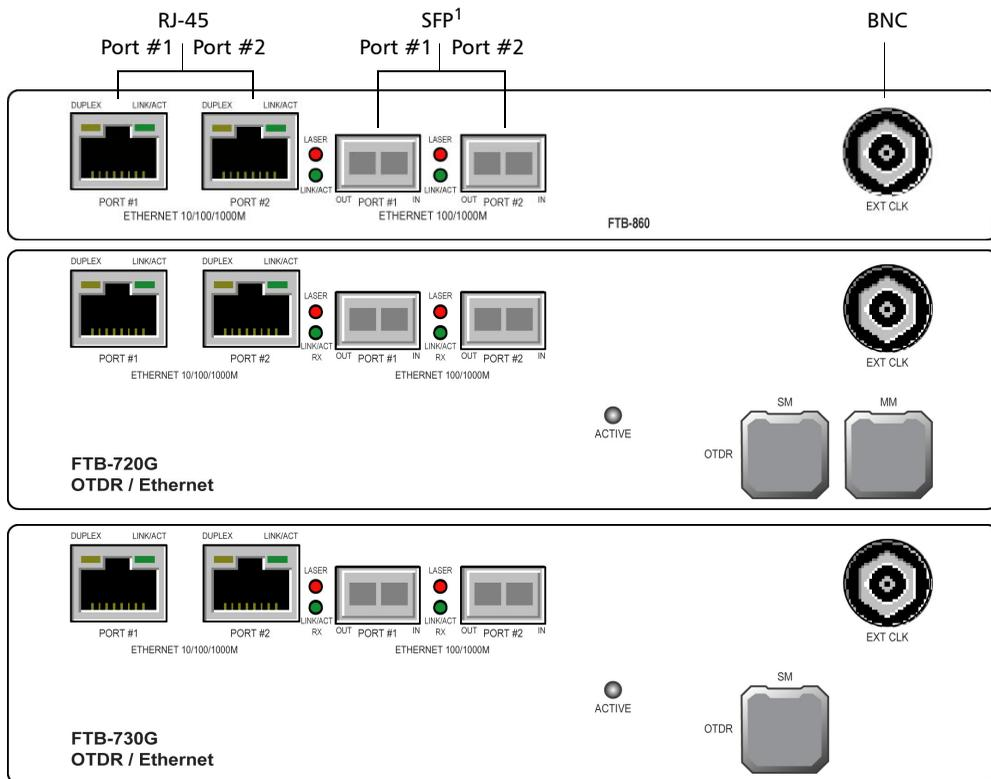
1. Laser radiation emitted from this port when LASER LED is on.
