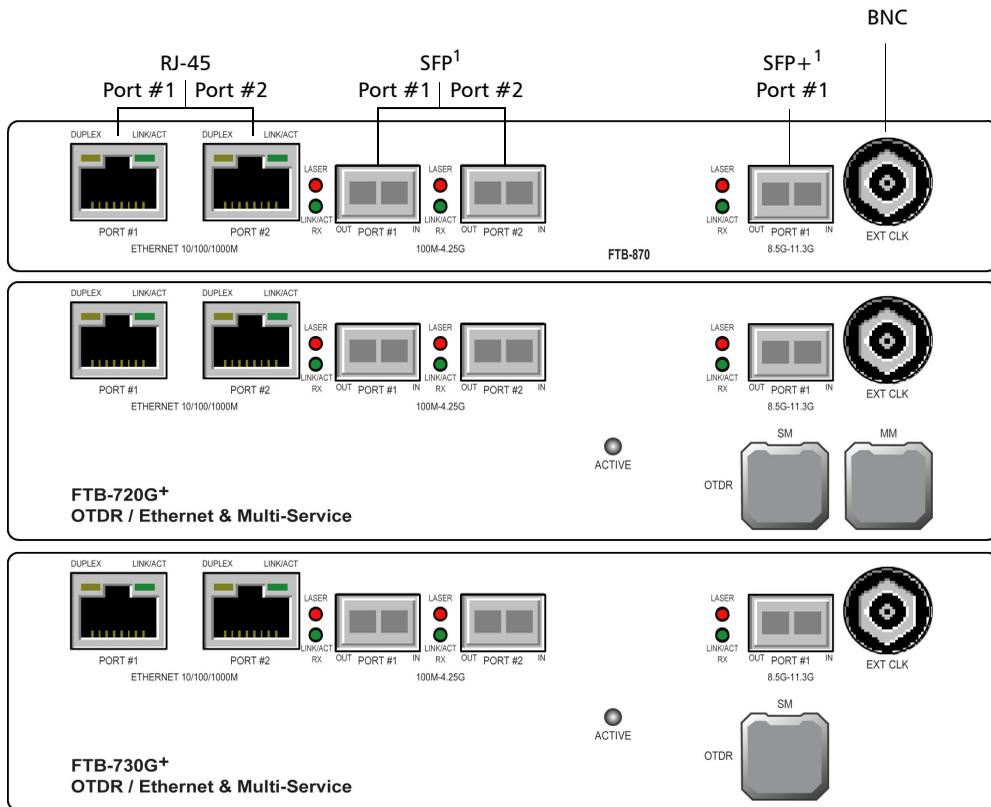
1. Laser radiation emitted from this port when LASER LED is on.
