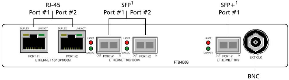
1. Laser radiation emitted from this port when LASER LED is on.
