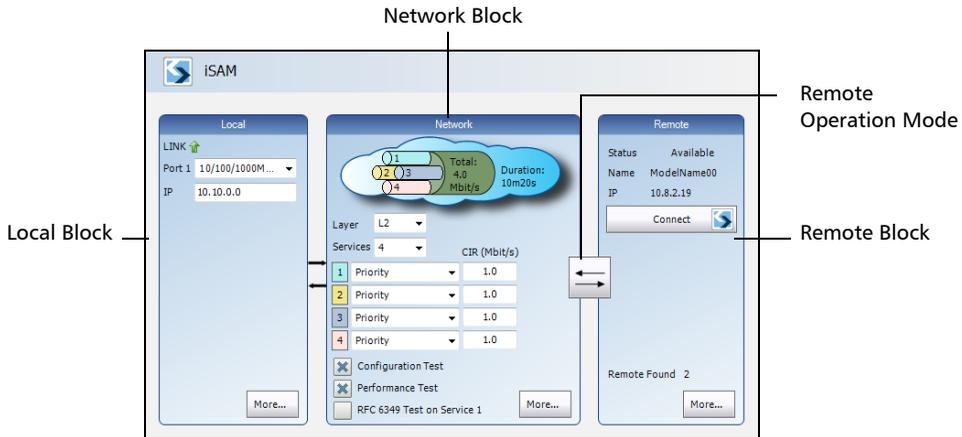
The block arrangement represents the network under test. From any block, either select the basic parameters or click on **More** for all settings.
