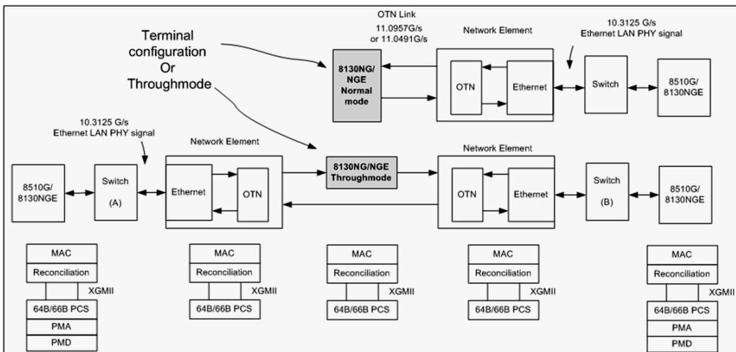
The Ethernet layer provides the equivalent functionality of the BERT Framed Layer 2 Test application supported on EXFO's Datacom product family with the particularity that there is no Ethernet Physical port as such. The Ethernet frame has its Ethertype field set to 0x88B7.
