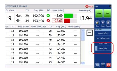
To view only the channels where power was detected, use the – button. To revert to the full channel view, use the + button.
