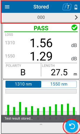
Test executed, 4 s to test again. Then go to next measurement.
