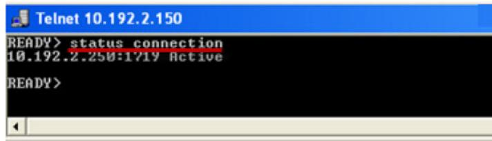
The screenshot shows a Telnet session window titled "Telnet 10.192.2.150". The command "status connection" is entered, and the response shows a connection with IP address 10.192.2.250:1719 in an Active state. The prompt "READY>" appears at the bottom.
