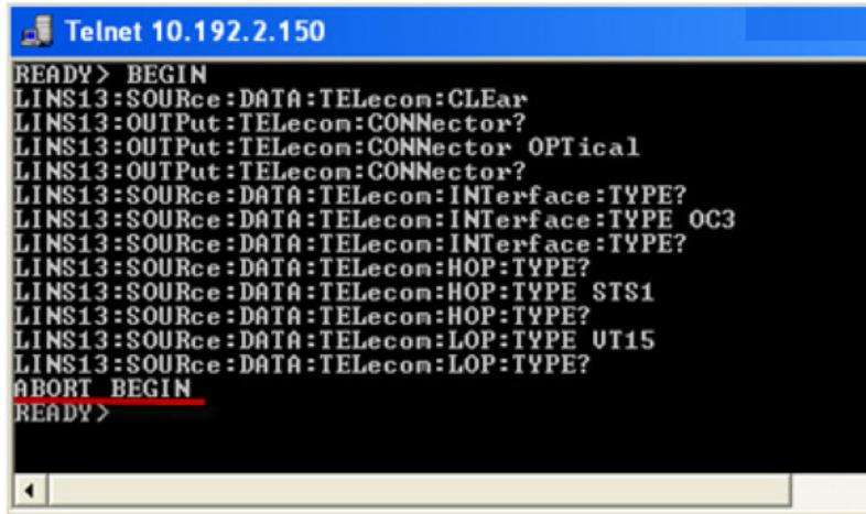
The screenshot shows a Telnet session connected to IP 10.192.2.150. The command history displays several SCPI commands related to telecom interfaces, all enclosed within a BEGIN...END block. The commands include source clear, connector types, and interface types. The word 'ABORT' is followed by 'BEGIN' in red, indicating it was part of the copied script. The session ends with 'READY>'.
