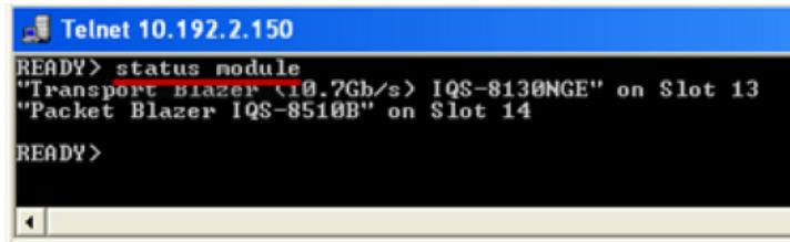
The screenshot shows a Telnet session window titled "Telnet 10.192.2.150". The command "status module" is entered, and the response displays two modules: "Transport Blazer (10.7Gh/s) IQS-8130NGE" on Slot 13 and "Packet Blazer IQS-8510B" on Slot 14. The prompt "READY>" appears at the bottom.
