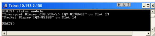
A screenshot of a Windows Telnet window titled "Telnet 10.192.2.150". The window shows the command "READY> status module" followed by the output: "Transport Blazer <10.7Gb/s> IQS-8130NGE" on Slot 13 and "Packet Blazer IQS-8510B" on Slot 14. The window has standard Windows controls (minimize, maximize, close) at the top right.
