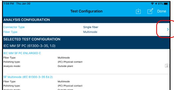
**6c.** In the **Analysis Configuration** window, tap **>** to change the connector type.
