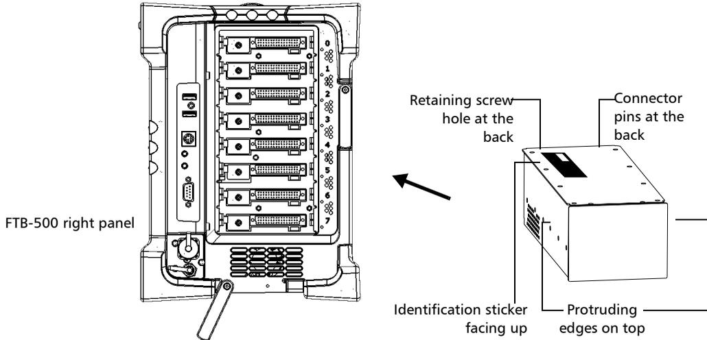
4. Insert the protruding edges of the module into the grooves of the receptacle's module slot.
