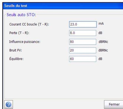
The screenshot shows a dialog box titled "Seuils du test" with a blue header. Below the header, the text "Seuils auto STO:" is displayed. The dialog contains five rows of configuration options, each with a text input field and a unit label:
