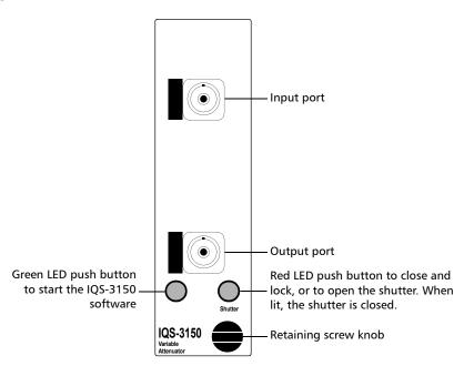
The module is configured for singlemode or multimode fibers and complies with optical return loss measurement (ORL) standards on transmission equipment.
