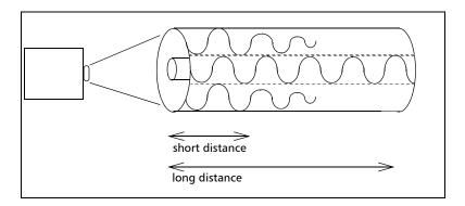
Due to the internal optics of the Variable Attenuator (and the majority of attenuators), most of the cladding modes are filtered out. This means that, with the attenuator connected, the power meter will display a loss greater than the attenuation setting of the attenuator (cladding modes have been partially stripped).
