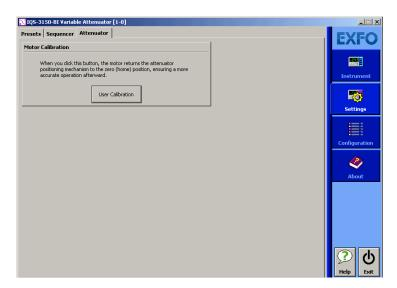
The attenuator mechanism is moved to the zero (home) position.
