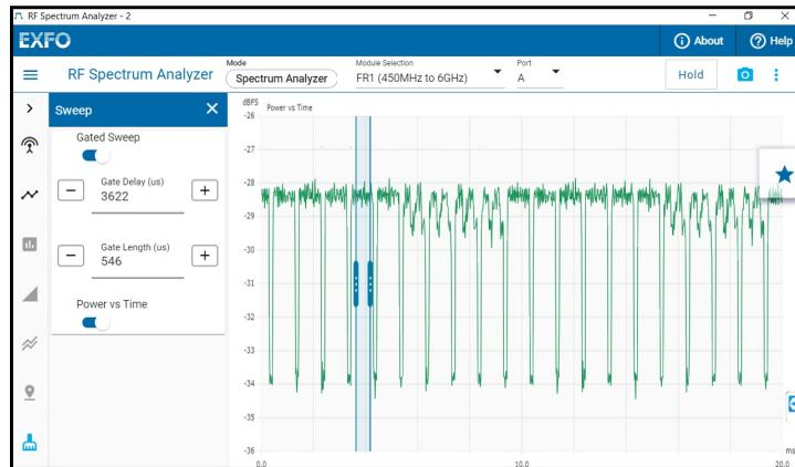
**Frame Duration (ms)** allows selecting the X axis length of the **Power vs Time** graph: **10 ms** (default) or **20 ms**.
