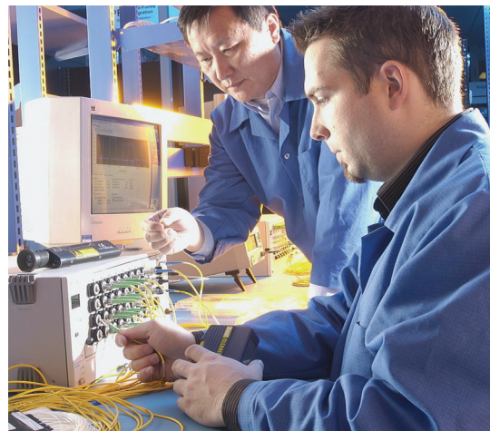
EXFO's IQS-12008 All-Band Component Analyzer performs IL, ORL and PDL measurements over a wavelength range of nearly 400 nm, for up to 32 channels simultaneously.
