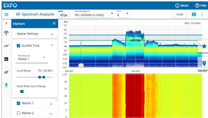
Figure 1. Real-time persistence spectrum and spectrogram.
