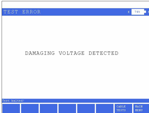
Figure 5.2.4A- Example of High Voltage Detection Screen
