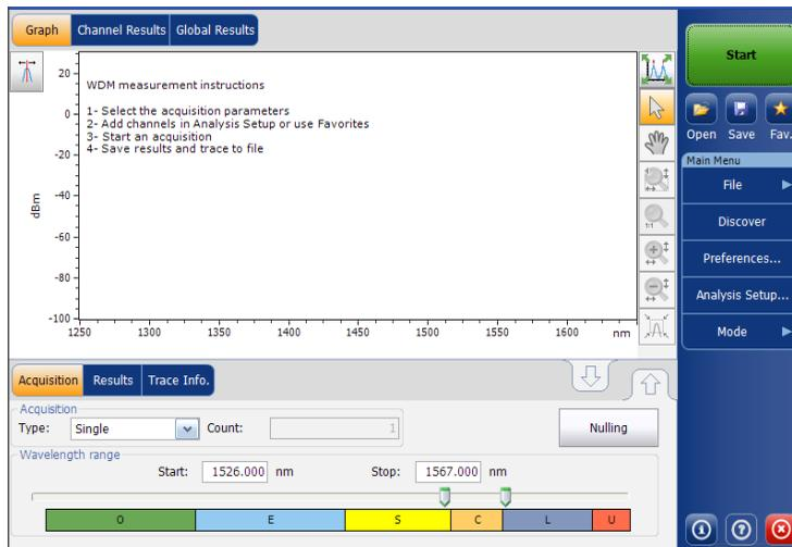
When the acquisition is taken (see *Starting a Measurement* on page 237 for details on how to perform a test), the active trace will be displayed in the tab with information along the following axis values:
