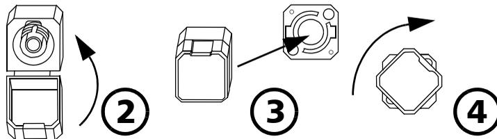
2. Close the dust cap in order to hold the connector adapter more firmly.
