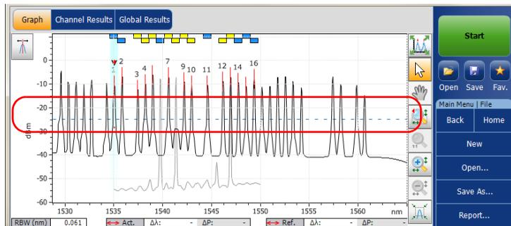
A peak detection level cursor is available in the graph when the **Results** tab is selected. The cursor is positioned along the Y-axis in accordance with the application's peak detection level global analysis parameter.
