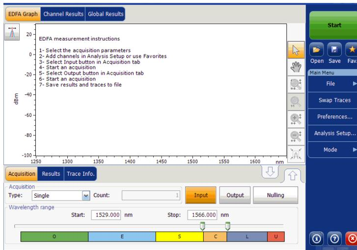
When the acquisition is taken (see *Starting a Measurement* on page 237 for details on how to perform a test), the trace will be displayed in the **EDFA Graph** tab with information along the following axis values:
