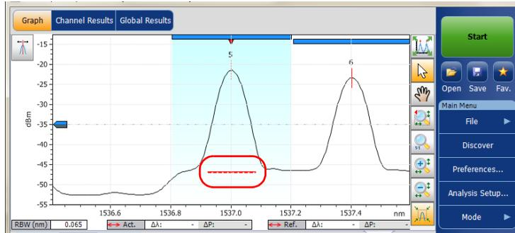
A dotted line across the full spectral width corresponds to the peak detection level indicator. This line indicates the minimum power level (dBm) from where a peak can be considered as a valid signal.
