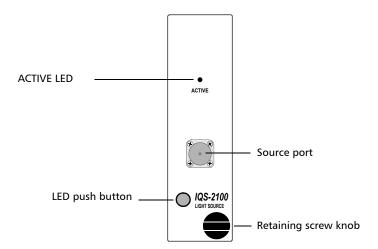
The IQS-2100 Light Source is designed for optimal stability. Steady drive circuitry maximizes optical output power and maintains excellent stability, while precision optical components ensure efficient, low-loss, narrow-beam output coupling. Laser sources are stabilized by thermoelectric Peltier coolers that regulate submount internal temperature.
