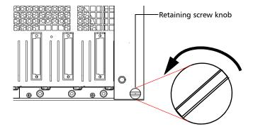
**2.** Place your fingers underneath the module or hold it by the retaining screw knob (*NOT by the connector*) and pull it out.
