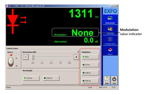
**2.** You can also select a modulation frequency from the QuickTools utility. For details, see *Monitoring Light Source Modules* on page 29.
