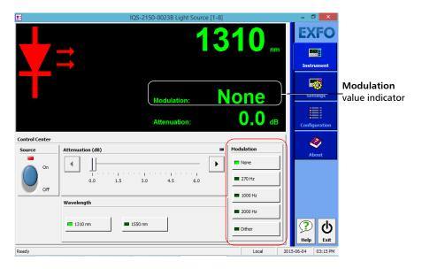
**2.** You can also select a modulation frequency from the QuickTools utility. For details, see *Monitoring Light Source Modules* on page 33.
