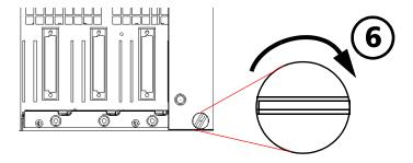
The module is correctly inserted when its front panel is flush with the front panel of the controller or expansion unit.
