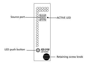
The IQS-2150 Light Source is designed for optimal stability. Steady drive circuitry maximizes optical output power and maintains excellent stability, while precision optical components ensure efficient, low-loss, narrow-beam output coupling.
